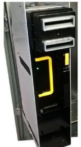
The other note unit provided by CI tech and installed in MFM31 at Highbury & Islington, has also suffered some teething problems, with notes being jammed in the unit and some communications issues caused by the connection to the unit being damaged as the unit was rotated for servicing.
