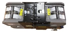
As mentioned above and outlined in TRU149, changes have been made to all of the MFMs at the stations shown above to allow station staff greater access to clear note jams when they occur within the Note Handling Unit (NHU).
